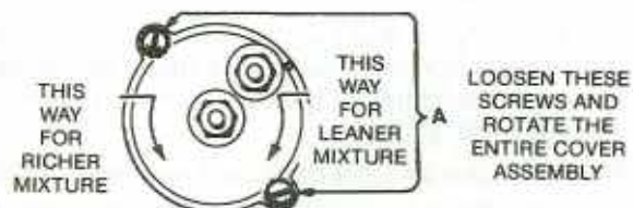
FIGURE 20. ELECTRIC CHOKE ADJUSTMENT
