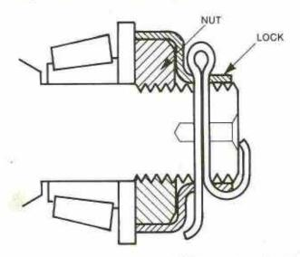
7a. On medium duty (I-50 thru I-80) axles, install lock over adjusting nut, aligning a slot in the lock with the hole in spindle for cotter pin. If slots will not align with hole, tighten nut to first position of alignment and install lock. Install cotter pin as shown.
