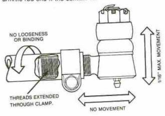
CAUTION—When tie rod or drag link ends are replaced, they must be threaded into the tie rod sufficiently so that when the clamp is applied, the clamping action will be directly over the threads on the ball joint end, as shown.
