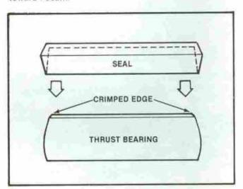
Position knuckle onto king pin boss of I-beam. Install lower seal over thrust bearing with crimped seam toward the seal.
