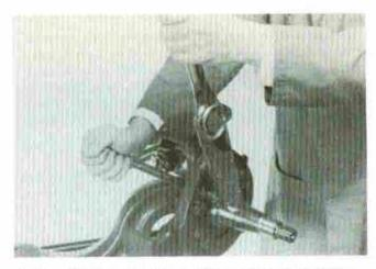
Reinstall brake backing plate or caliper mounting bracket. Torque mounting nuts to 110-120 ft. lbs. (149-163 N·m) on the medium duty axles and 220-240 ft. lbs. (298-325 N·m) on the heavy duty alxes.
