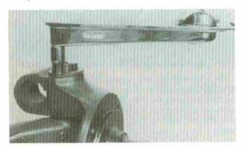
Install king pin end caps and O rings. Torque bolts to 12-16 ft. lbs. (16-22 N-m).
