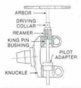
Line ream the new bushings to finished dimensions shown in specifications.
