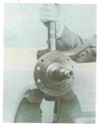
Remove the old bushings, using an arbor or drift with proper adapter so damage to bore in spindle does not occur.
