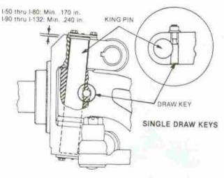
3. Install draw keys. The single draw keys are installed with the nut and lock washer to the front side of the axle. Torque to 25-30 ft. lbs. (27-37 N-m). Tap unthreaded end of draw key sharply with a hammer and retorque the draw key nut.
