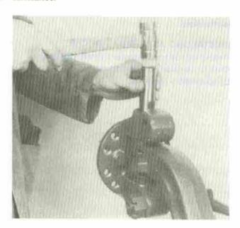
2. Prelube lower half of king pin with clean chassis grease. Align draw key flats with holes in I-beam and install king pin into upper spindle bore by hand, until It passes thru the bushing, upper seal, and shims. If king pin does not pass through freely to the I-beam, it must be removed and components re-aligned. After king pin starts through I-beam, a brass drift and hammer maybe used to assist installation.
