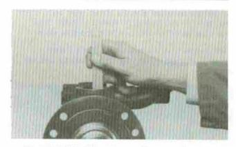
Be certain thrust bearing and lower seal are positioned properly. Center king pin vertically in the knuckle, with minimum of .240 inch distance from top machined surfaces of knuckle on Models I-90 thru I-132 and .170 inch on Models I-50 thru I-80. This allows proper clearance for king pin end cap installation,
