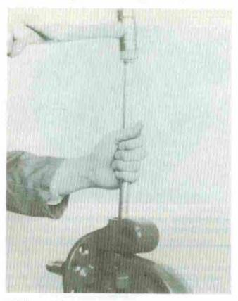
Drive out king pins, using a soft hammer and drift.CAUTION: Do not heat I-beam end to aid removal of king pins.
