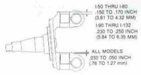
2B. When replacement bushings are 1.500 inch (38.10 mm) long composite, the measurements are taken from the top machined surfaces of the knuckle as shown above.
