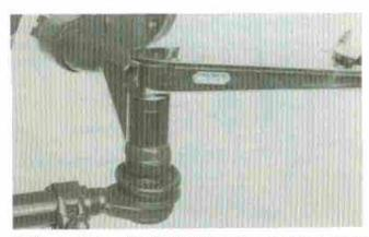
7. Reinstall tie rod ends into tie rod arms and torque to 85-105 ft. lbs. (115-140 N-m) minimum on I-50 thru I-80 axle, and 140-160 ft. lbs. (190-215 N-m) minimum on I-90 thru I-132 axle. If cotter pin cannot be installed after minimum torque is attained, the nut must be tightened until cotter pin can be installed.
