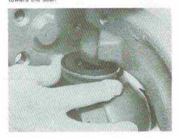
Install bearing and seal between I-beam and knuckle with seal up.
