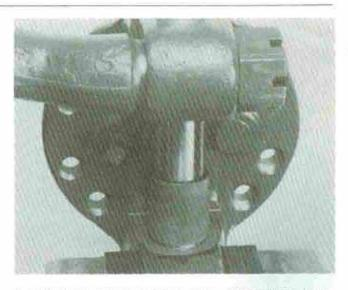
Install upper grease seal into knuckle with lip down toward I-beam.
