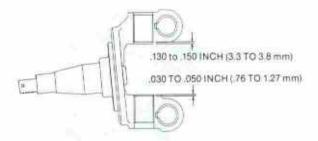
2A. The dimensions shown above are used when replacement bushings are full length. The measurements are taken from the machined surface of the knuckle that borders the king pin boss of l-beam (top) and the thrust bearing (bottom).
